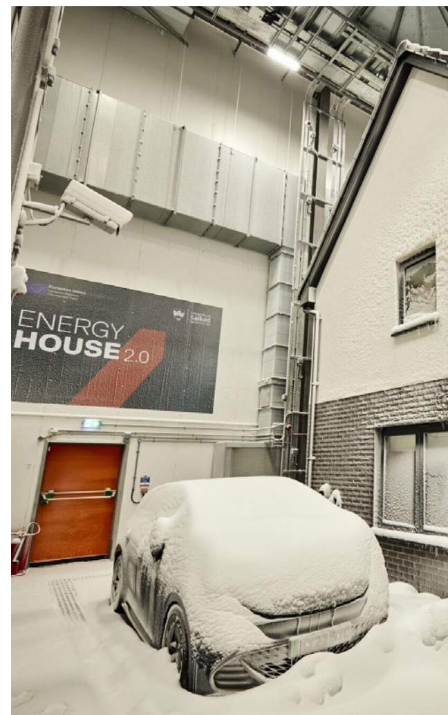
The eHome2, built with the Energy House 2.0, which can simulate temperatures ranging between -20°C to +40°C, and wind, rain, snow, and solar radiation.
